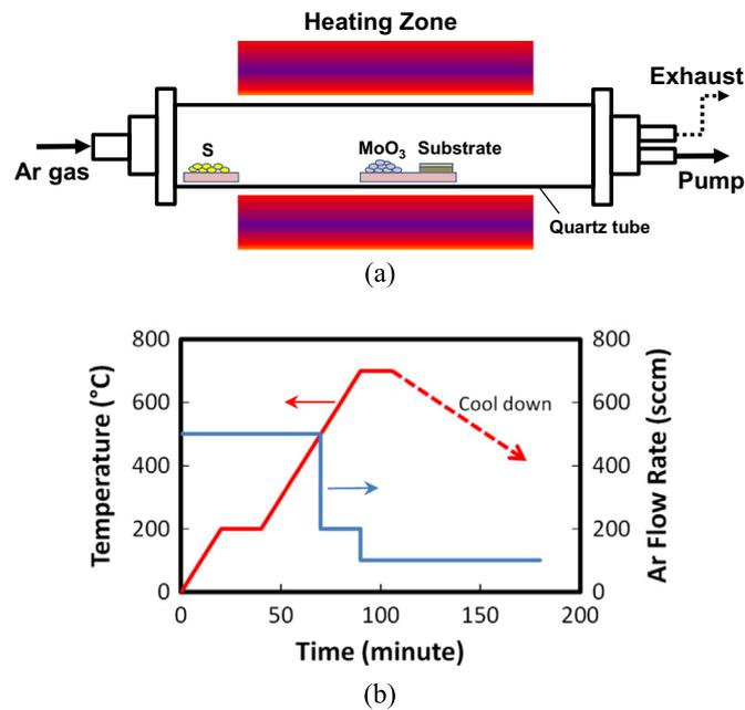
**Fig. 1.** (a) Schematic diagram of the CVD system for MoS<sub>2</sub> atomic layer growth; (b) temperature and gas flow programming during the chemical synthesis.
