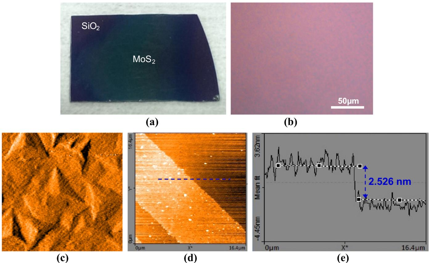
**Fig. 2.** Synthesized MoS<sub>2</sub> film on a SiO<sub>2</sub>/Si substrate with (a) optical photograph with clear color contrast between MoS<sub>2</sub> and SiO<sub>2</sub>, (b) microscopic image of MoS<sub>2</sub> film, and AFM images of MoS<sub>2</sub> crystals (c) in triangle shape before growth improvement, (d) forming a continuous film after improvement of growth parameters, and (e) thickness profile of a tri-layer MoS<sub>2</sub> film.
