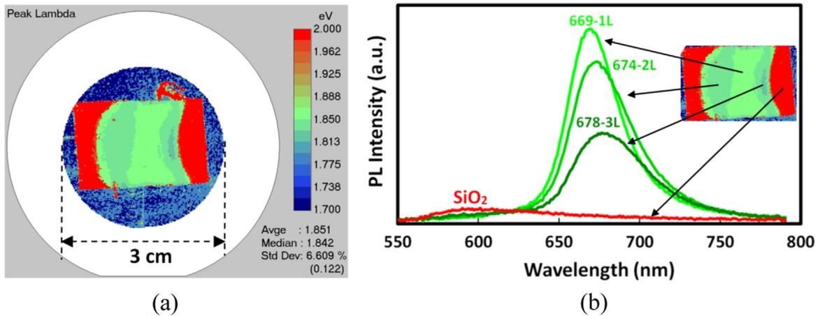
**Fig. 3.** PL characterization of synthesized MoS<sub>2</sub> films grown on a SiO<sub>2</sub>/Si substrate. (a) PL mapping with a scanning spatial resolution of 200 μm × 200 μm across the substrate. (b) PL spectra from 4 different areas on the substrate showing layer numbers and thickness dependence of the PL intensity.
