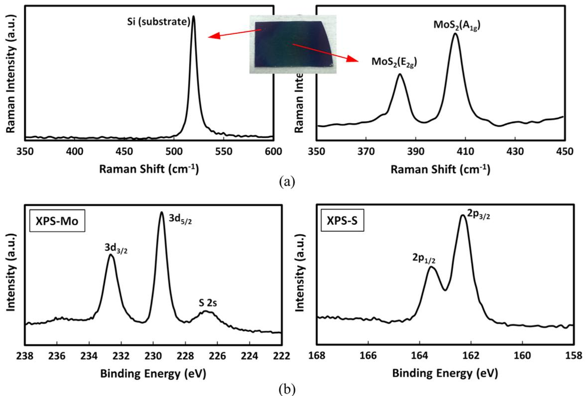
**Fig. 4.** (a) Raman spectra of Si substrate and synthesized tri-layer MoS<sub>2</sub> on the substrate with two peaks positioned at 383.6 cm<sup>-1</sup> and 405.7 cm<sup>-1</sup>, corresponding to the E<sub>2g</sub> and A<sub>1g</sub> vibration modes, respectively. (b) XPS scan of the synthesized MoS<sub>2</sub> film with binding energy of Mo 3d at 229.5 eV and 232.6 eV, and S 2p at 162.3 eV and 163.6 eV.
