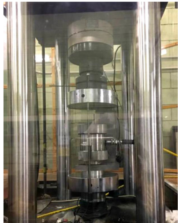
Fig. 1. Instrumentation and test setup used in compression tests.
