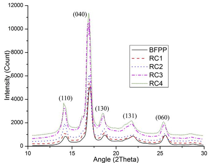
Fig. 6. XRD pattern for composite specimens.
