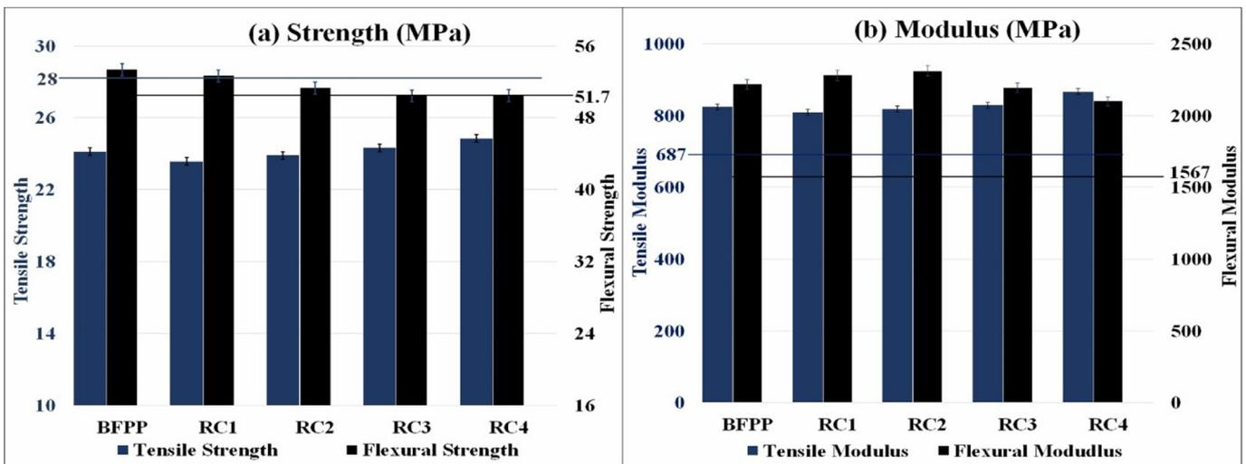
Fig. 4. Mechanical properties of fresh and recycled composites (a) Strength (b) Modulus.
