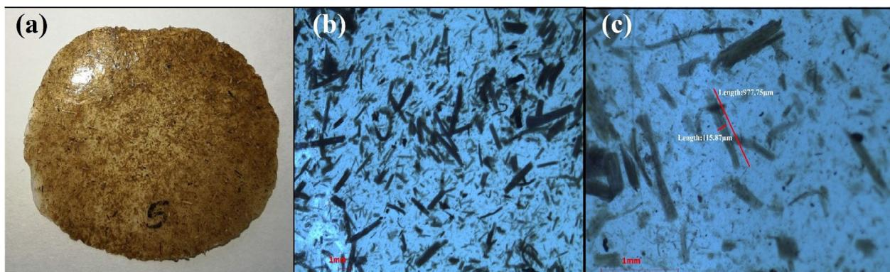
Fig. 2. (a) Thin film of composite (b) at 5 $\times$  magnification (c) at 50 $\times$  magnification.
