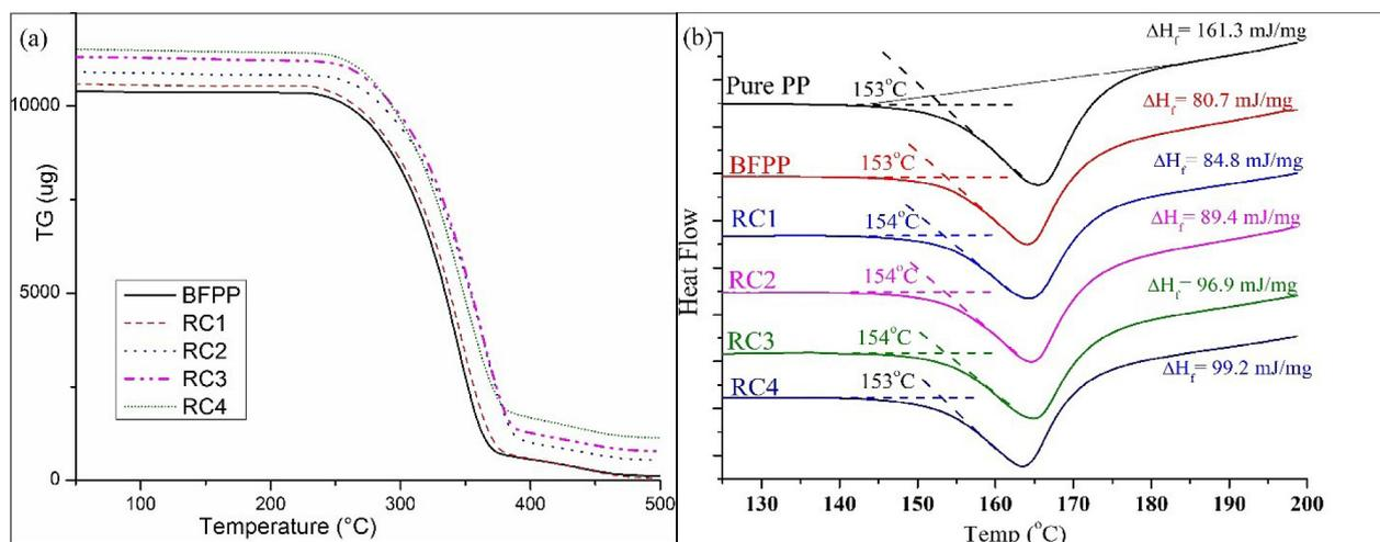
Fig. 5. (a) TGA Curve and (b) DSC curve for fresh and recycled composites.
