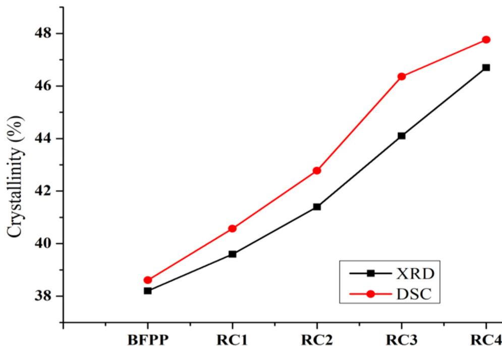
Fig. 7. Crystallinity of composite specimens by XRD and DSC methods.
