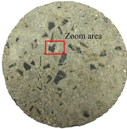
(a) The cross section diagram of the rubber particle mortars sample.
