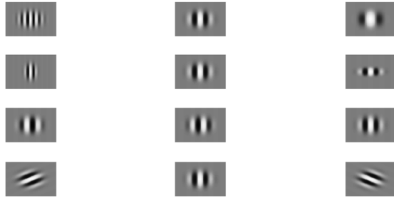
Figure 3. 2D Gabor filters. Rows (from bottom to top ) show the distinct effects of bandwidth, aspect ratio, phase offset and orientation, respectively.
