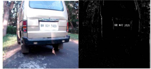
Figure 7[14]. Original image (left) and result of vertical Gabor filter based edge detection (right)
