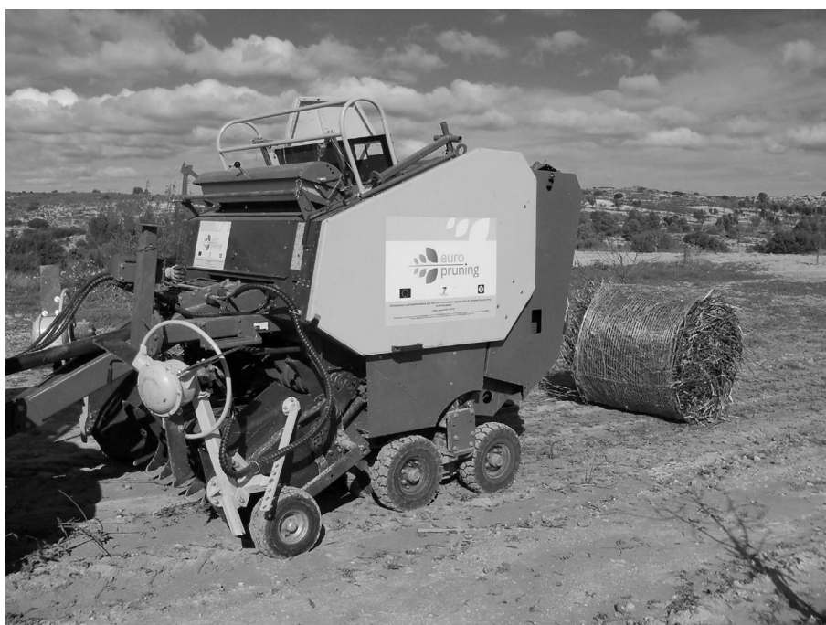
Fig. 3. Innovative pruning baler developed by PIMR (mod. PRB 1,75) during the European project Europruning [23].
