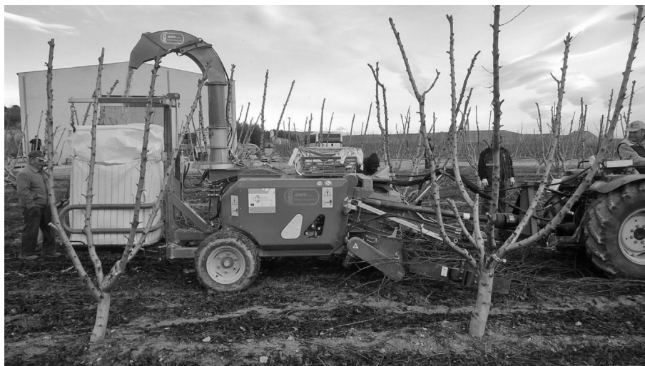
Fig. 2. Innovative pruning chipper developed by ONG (mod. PC50) during the European project Europruning [23].
