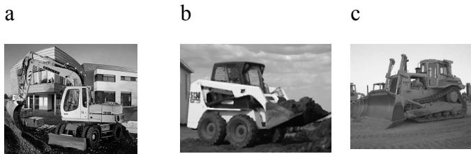
Fig. 1: Examples of construction machinery: a) excavator, b) skid-steer loader, and c) bulldozer.
