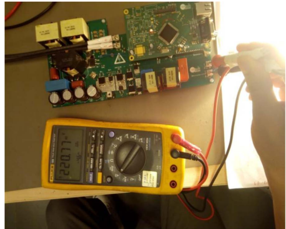
Fig. 21. Output voltage of the micro-inverter measurement.
