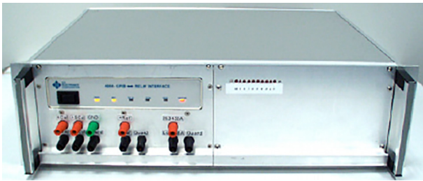
Fig. 1. External view of the INRIM divider instrument. A 19" case holds two copper boxes, one with the resistive divider and the other with the relays system, a GPIB I/O interface and the power supply.
