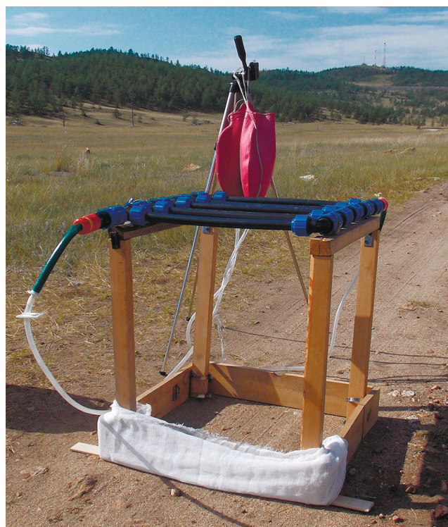
Fig. 2. Rainfall simulation device applied in the study.
