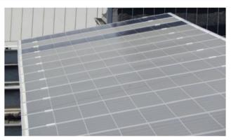
Fig. 1 An experimental set-up for in situ natural dust deposition on the photovoltaic modules
