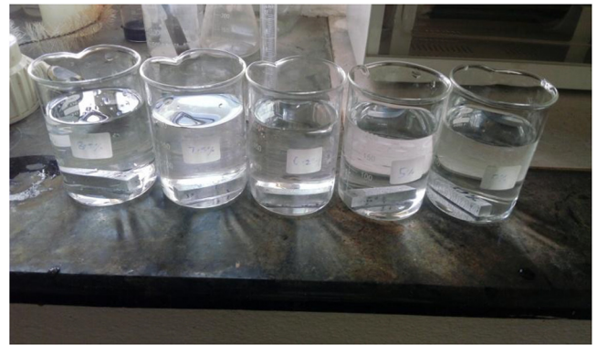
Fig. 8. Immersion corrosion test samples for different AA5083/MWCNT compositions.
