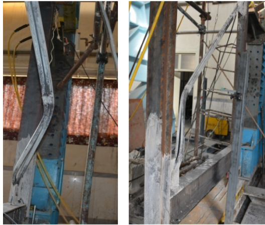
Figure 8. Large post buckling deformations in Test 2
