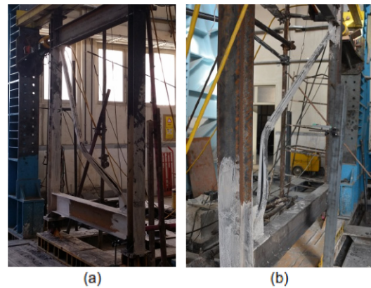
Figure 13. Deformations of braces (a) Test 1 (b) Test 2.
