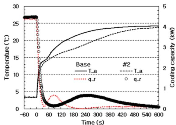
Figure 10. Comparison of coldness release capacity between Base and CSH ( $T_{amb} = 24\text{ }^{\circ}\text{C}$ ,  $Q = 450\text{ m}^3/\text{h}$ ).
