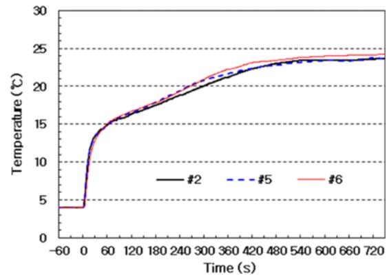
Figure 5. Experimental results of coldness release using various PCMs.
