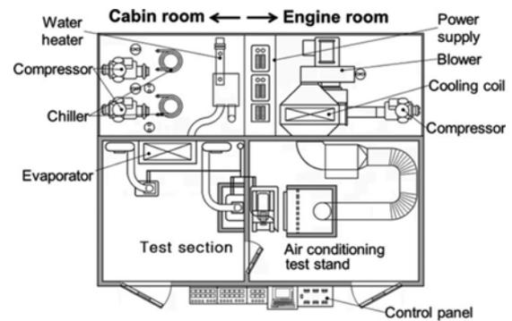
Figure 3. Schematic diagram of cold storage air-conditioning system test apparatus.
