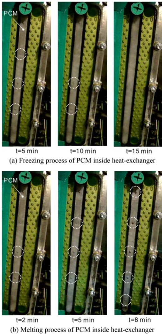
Figure 8. Visualization of freezing and melting process inside cold storage heat exchanger.
