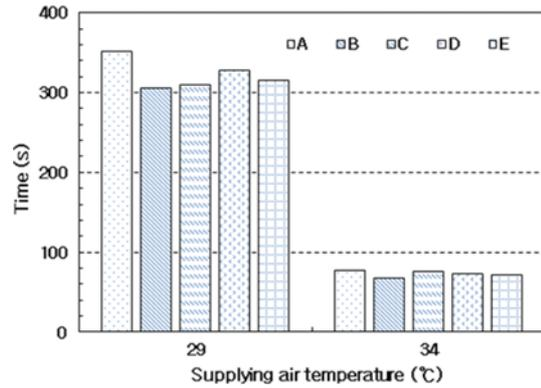
Figure 7. Comparison of 24 °C air discharge temperature under various ambient temperatures ( $Q = 450\text{ m}^3/\text{h}$ ).
