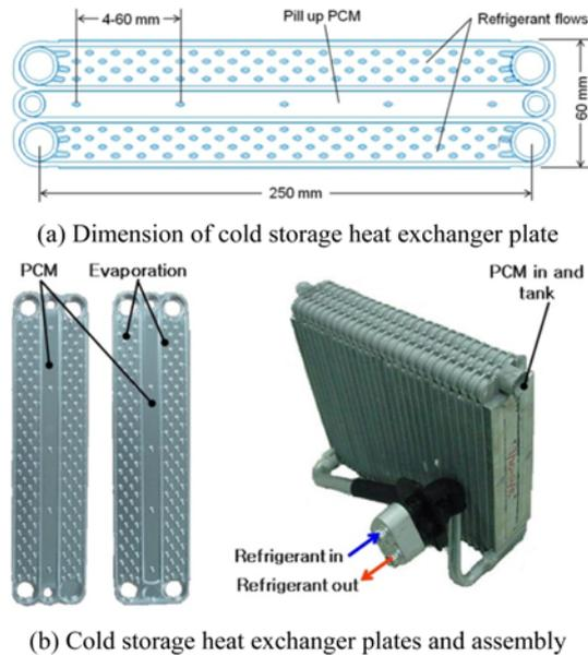
Figure 2. Photo of cold storage heat exchanger.
