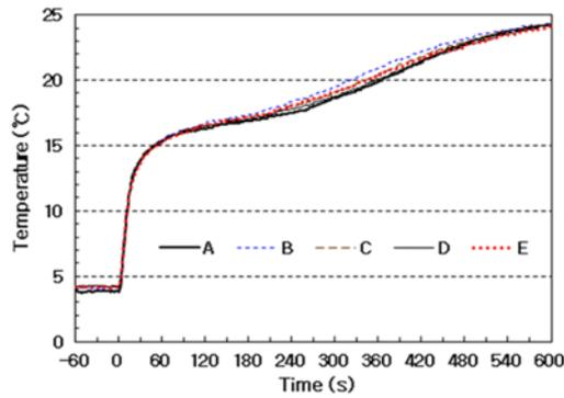
(a) Discharge air temperature ( $T_{amb} = 24\text{ }^{\circ}\text{C}$ ,  $Q = 450\text{ m}^3/\text{h}$ )
