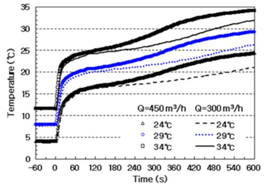
Figure 9. Coldness release performance with various air temperatures and air flow volume rates.
