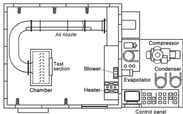
Figure 1. Schematic diagram of cold storage heat exchanger calorimeter.
