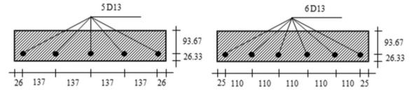
Fig. 2 Detail of reinforced concrete one-way slabs
