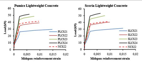
Fig. 7 Load-midspan reinforcement strain diagrams
