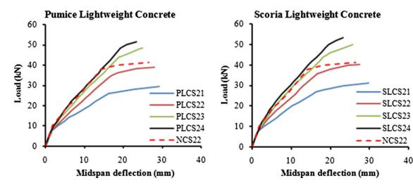
Fig. 5 Load-midspan deflection diagrams
