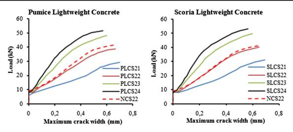
Fig. 6 Load-maximum crack width diagrams
