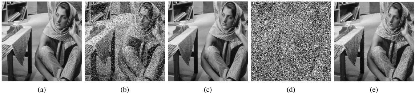
Fig. 6: Barbara image: (a) actual image, (b) at 20% noise, (c) filtered image; (d) at 80% noise, (e) filtered image.
