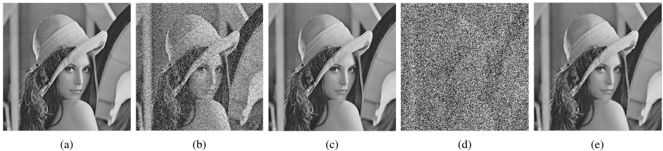
Fig. 7: Lena image: (a) actual image, (b) at 20% noise, (c) filtered image; (d) at 80% noise, (e) filtered image.
