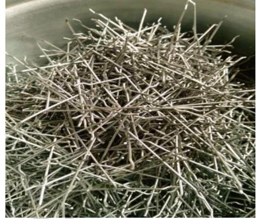
Figure (2): Sample of Steel Fiber
