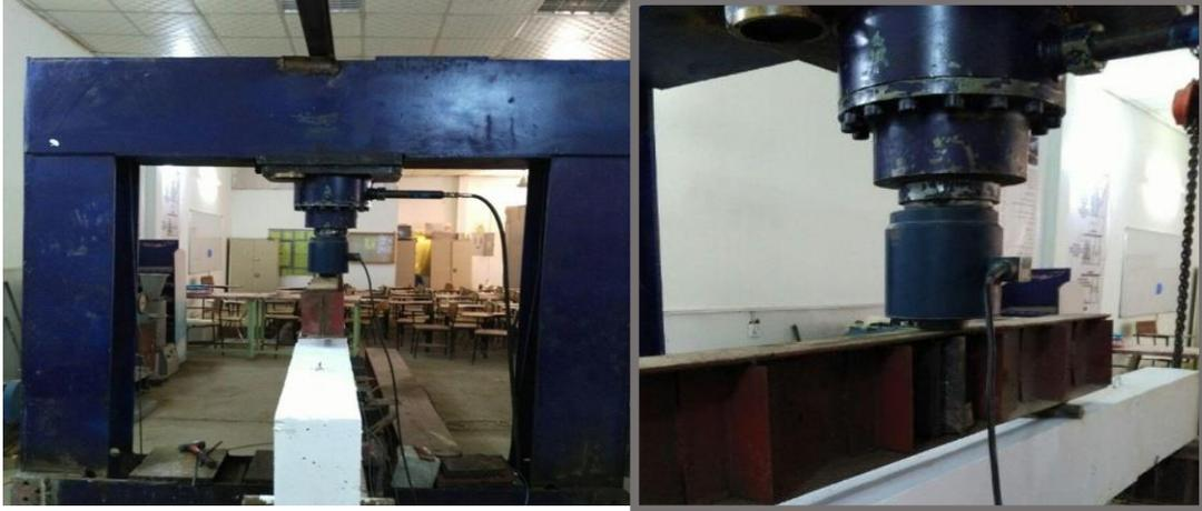
Fig. (6): Hydraulic Testing Machine of Concrete Girder Specimens
