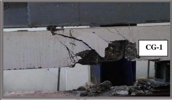
(b) GirderCG-1(direct shear & splitting of concrete covers)
