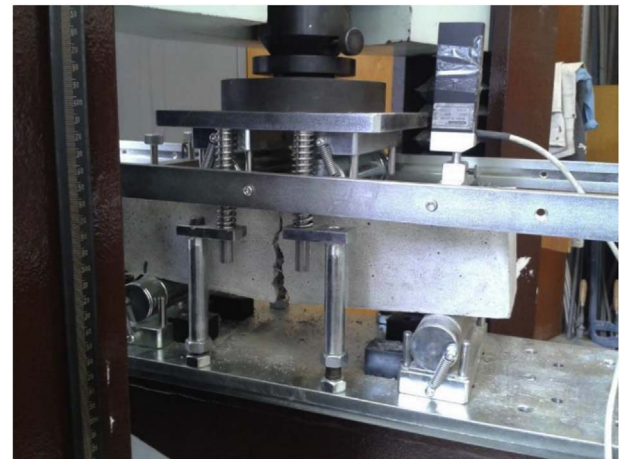
Fig. 6. 100 × 100 × 400 mm beam in testing machine.
