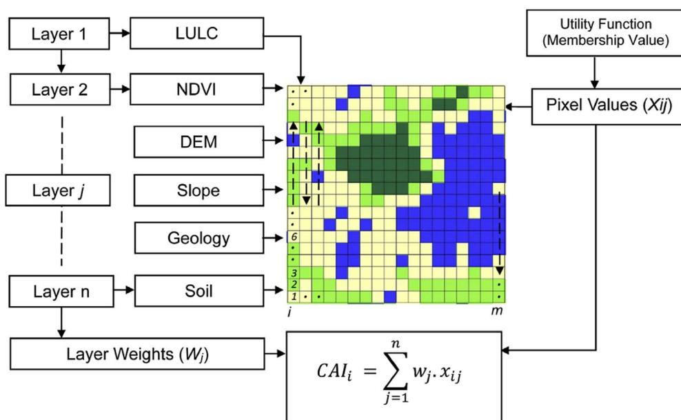
Fig. 3. Model description for computing Coastal Area Index in GIS.
