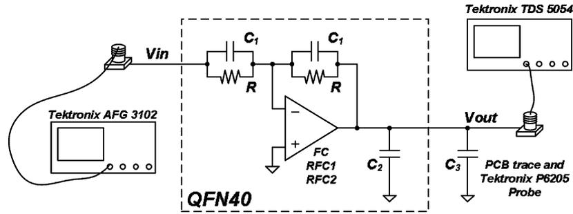
Fig. 5. Amplifier characterization setup used to measure the performance of the amplifiers.
