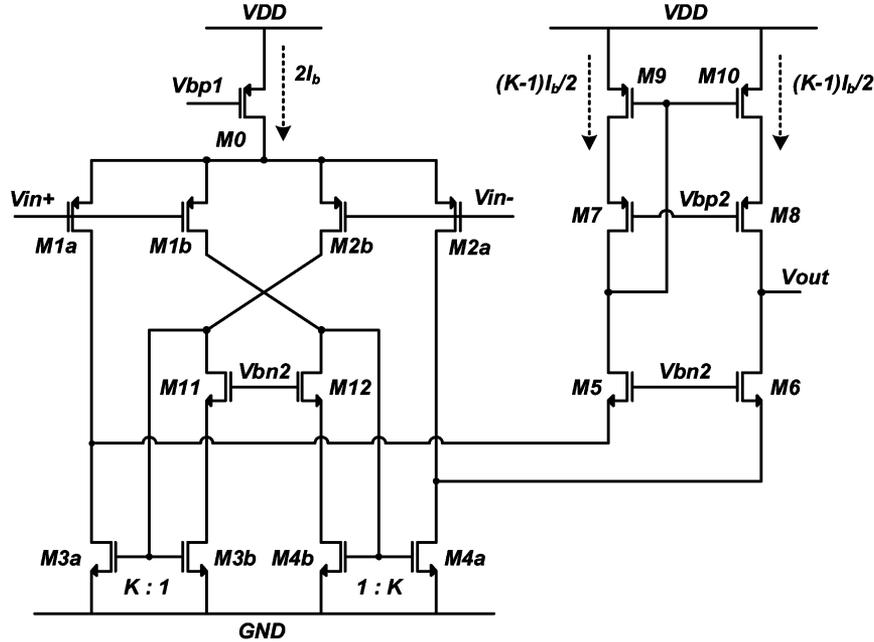
Fig. 2. The recycling folded cascode (RFC) amplifier.
