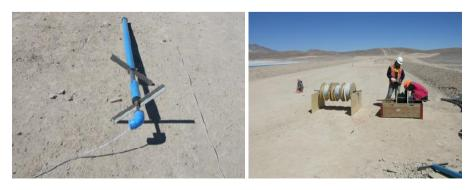
Figure 12: Special packaging for SOFO sensor and cable installation
