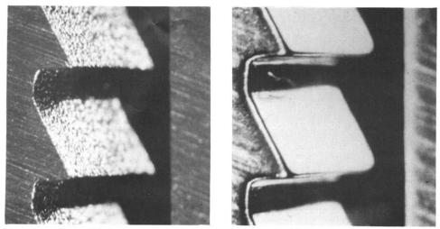
Figure 14 Figure 15 Close-up of the teeth on the extrusion die in Figure 13 shown before and after processing.
