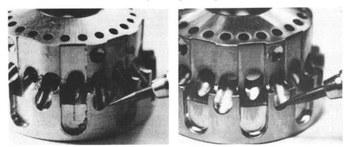
Figure 9 Figure 10 Turbine engine fuel spray nozzles use AFM to satisfy critical deburring requirements.
