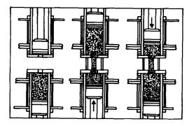
Figure 1 - Abrasive Flow Machining Process
