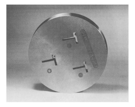
Figure 13 - Multiple passages in one workpiece can be processed simultaneously.
