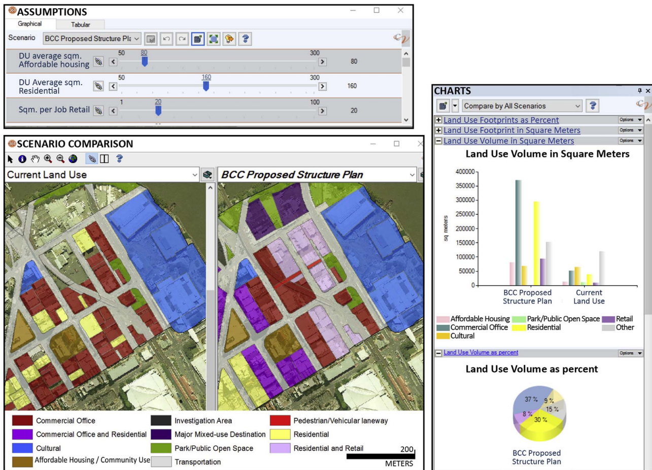
Fig. 5. CommunityViz ® slider bars allow users to input assumptions, which are used to generate comparisons between current conditions and proposed changes (shown here in 2D maps and bar graphs).
