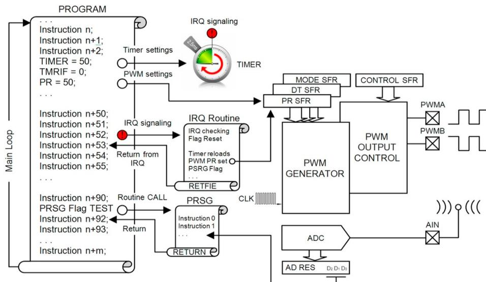
Fig. 3. Workflow of the DPWM control loop and pseudo randomly spread frequency generator.
