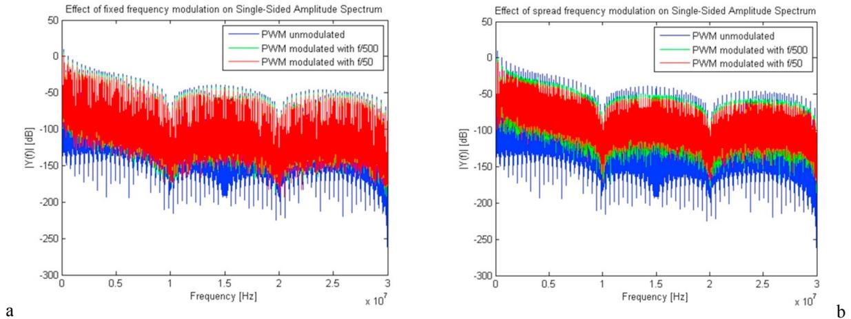
Fig. 4. (a) Fixed frequency modulation (b) Randomly spread frequency modulation.
