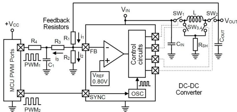
Fig. 1. Block schematic of the digitally controlled power supply unit pointing the key components of the system.
