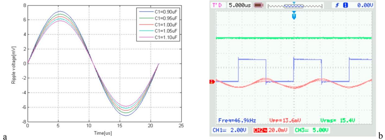
Fig. 2. (a) The ripple voltage on C1 depending its value (b) The measured ripple with 50% duty of DPWM.
