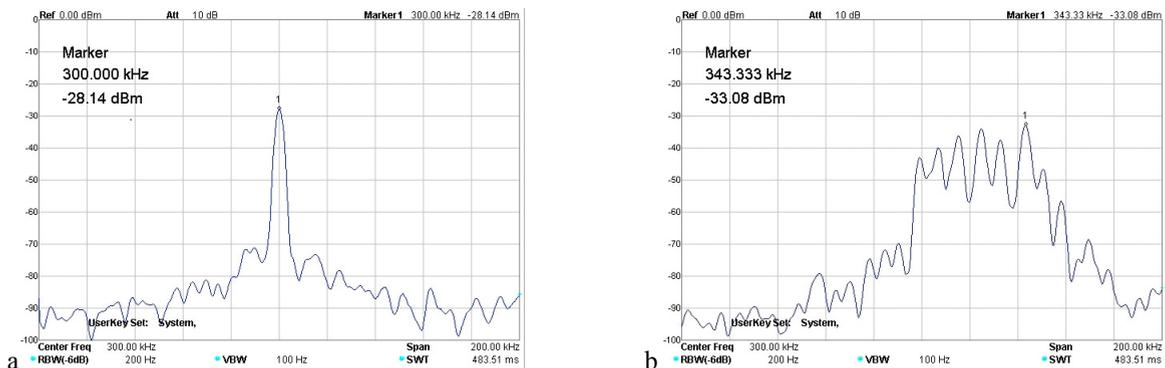
Fig. 5. (a) Switching noise without spread modulation (b) Switching noise with spread modulation.
