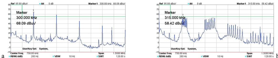
Fig. 6. (a) Switching noise without spread modulation (b) Switching noise with spread modulation.
