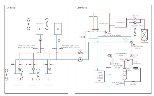
Fig. 2. The Scheme of VRF air conditioning system.
