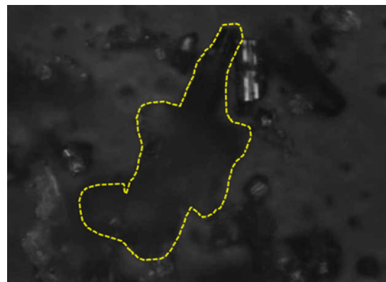
Fig. 12 Adhesive interface surface at the laminate angle of 30°
