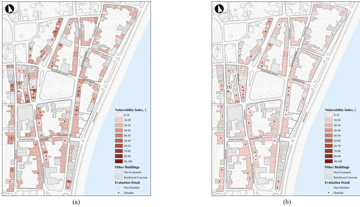
Fig. 9 Vulnerability index, I_v , obtained for: (a) BR condition and (b) RP3 retrofitting package
