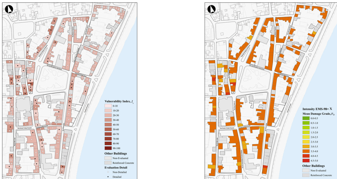
(a) BR building condition for macroseismic intensities I_{EMS-98} = IX and I_{EMS-98} = X
