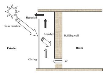
Fig. 7. Schematic diagram of solar chimney.
