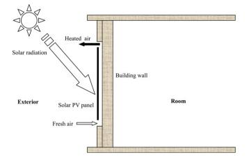
Fig. 4. Schematic diagram of building integrated photovoltaic system.
