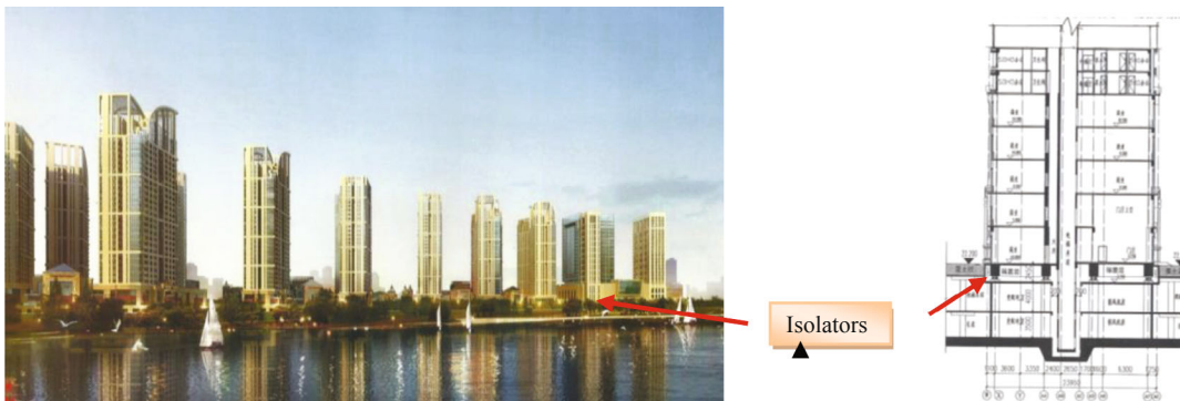
Fig. 10 24 high rise (31 stories) seismically isolated residential apartment buildings with floor area 980,000 m 2
