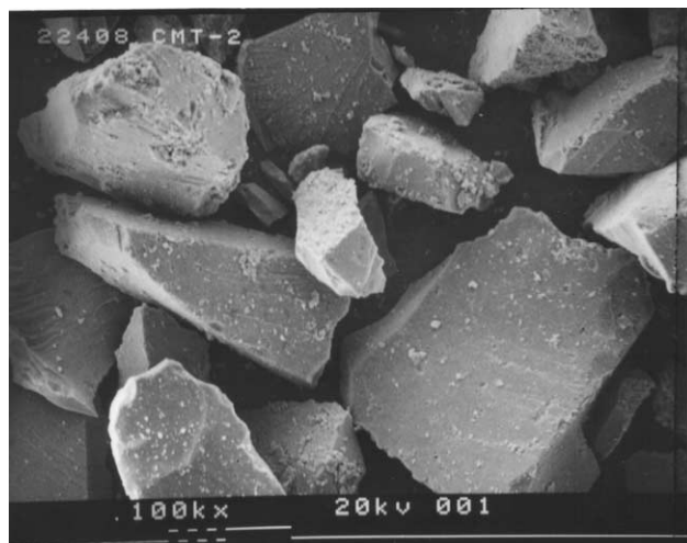
Fig. 2. Transmission electron microscopy photograph of the coke isolated from the \text{Fe}_3(\text{CO})_{12} containing upgrading reactions. Same conditions as Table 1.
