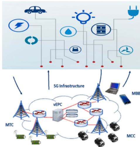
Figure 7: Example of 5G-IoT architecture [7, 12]
