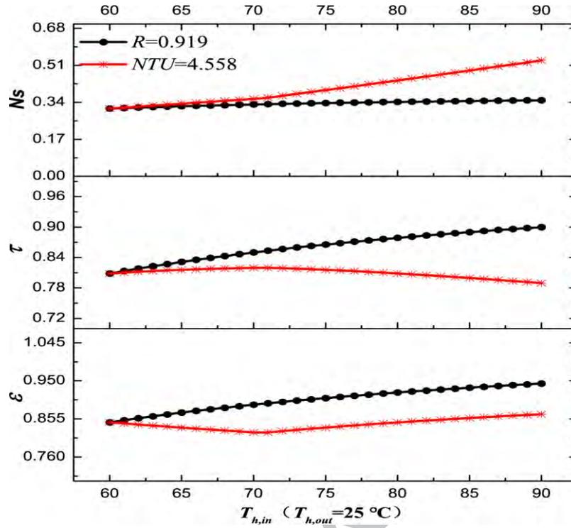
Fig.8 The variation of  $\epsilon$ ,  $\tau$  and  $N_s$  with  $T_{h,in}$  when selecting  $T_{h,out}$  as controlled variable
