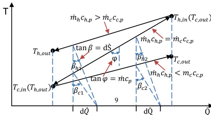
Fig.2  $T$ - $Q$  diagram for the counter flow heat exchanger ( $NTU \rightarrow \infty$ )
