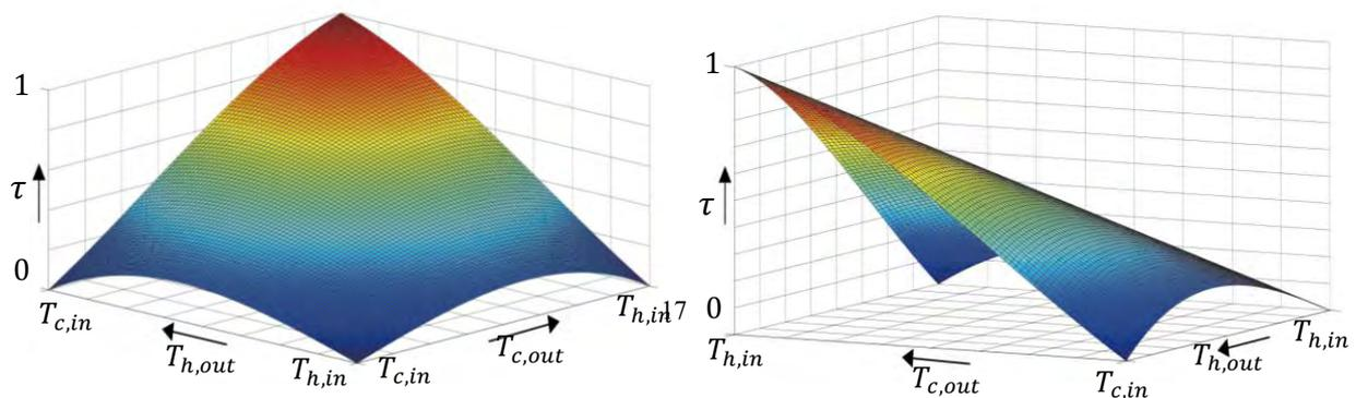
Fig.5 The change characteristics of  $\tau$  with  $T_{h,out}$  and  $T_{c,out}$
