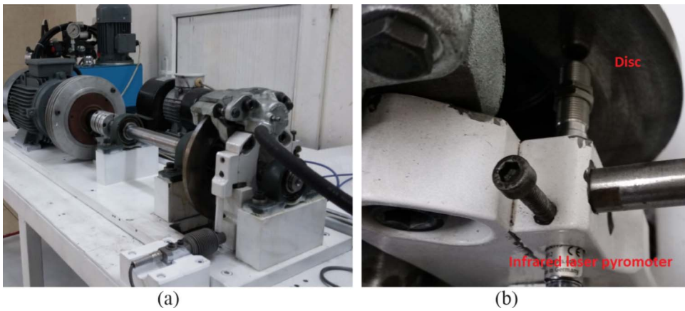
Fig. 3. Brake pad friction tester working in contact conditions: (a) overall view of components (b) view of attached IR pyrometer.
