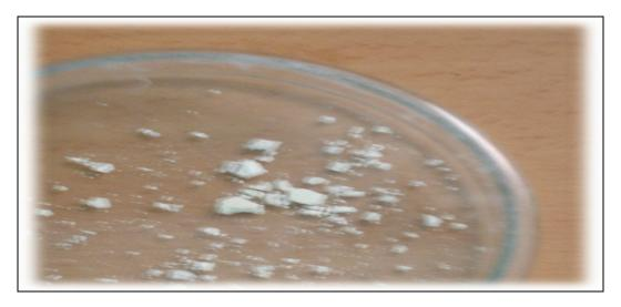
Fig.-1: Picture of synthesized Zinc Oxide nanoparticles
