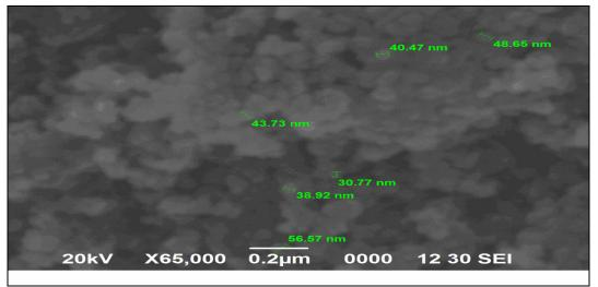
Fig.-2(a): SEM images of ZnO nanoparticles
