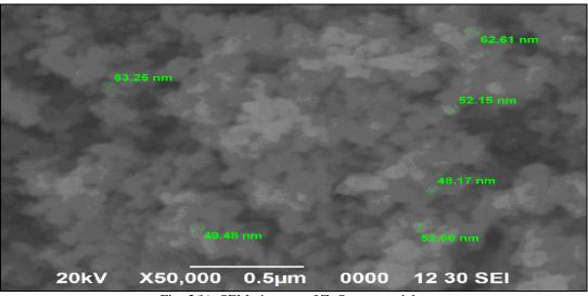
Fig.-2(b): SEM images of ZnO nanoparticles
