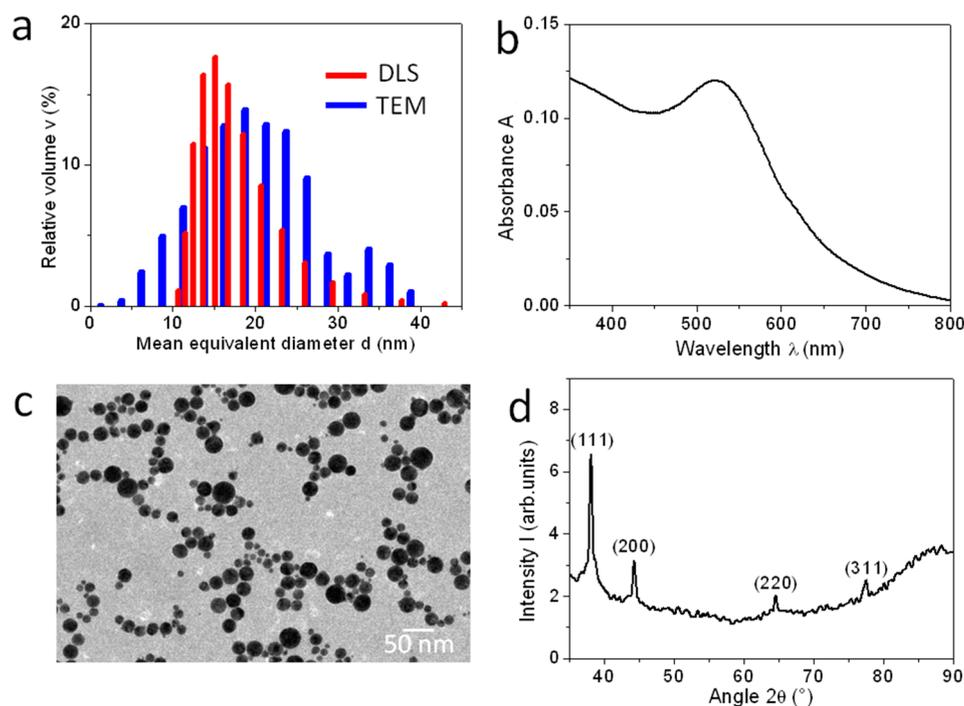
**Figure 1.** (a) Size measurements of the NPs resulting from LA of an Au target, from both DLS of the colloidal solution and analysis of TEM image after drop-casting on silicon substrate; (b) UV-vis absorption of the colloidal solution; (c) TEM image showing the size of the NPs in the direct space; (d) XRD pattern resulting from a sample of drop-cast Au NPs.
