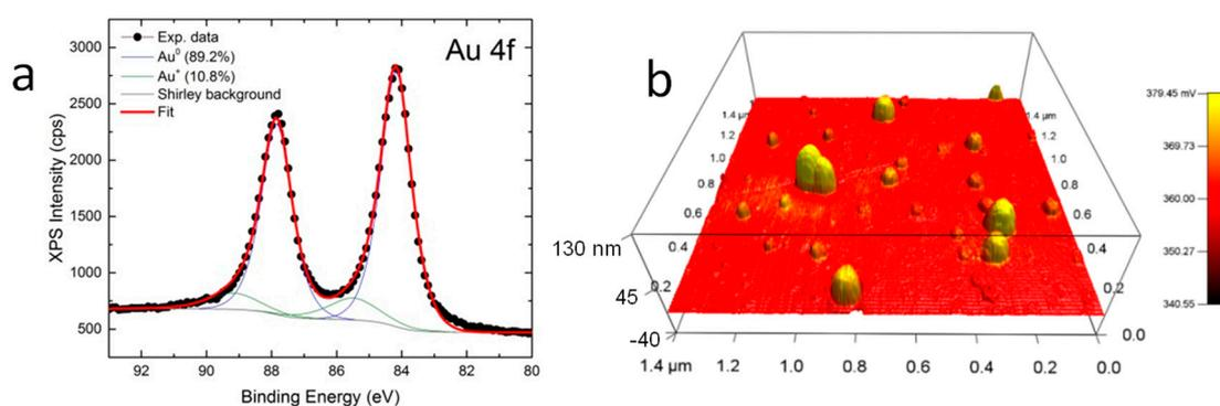
**Figure 2.** (a) XPS measurement of the Au NPs drop-cast onto HOPG, showing the presence of oxidized Au together with metallic Au; (b) AFM 3D image of topographic profile of the NPs on silicon, with electrical surface potential overlaid as the color levels.
