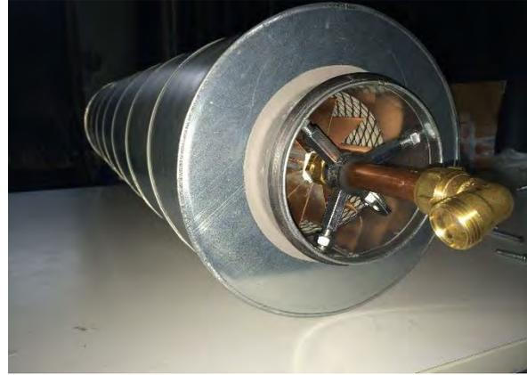
Figure 11: prototype integrated into duct silencer
