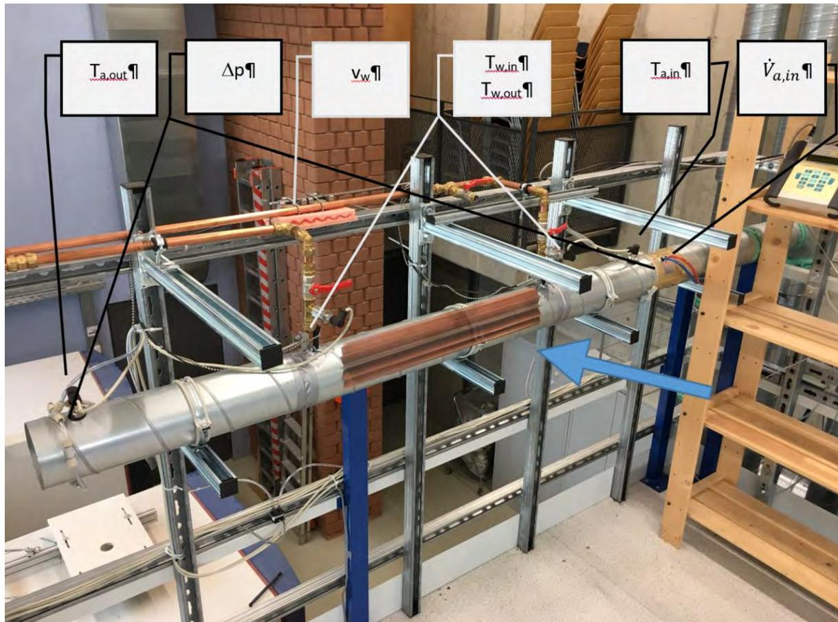
Figure 12: Placing the measuring sensors from Table 2 in the experimental setup
