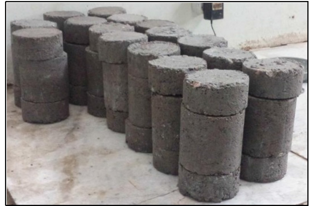
Fig. 2. Cylindrical specimens prepared for water absorption, sorptivity and electrical resistivity tests.
