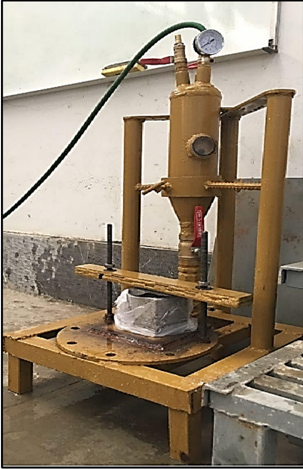
Fig. 4. Device prepared to perform the water penetration depth test.
