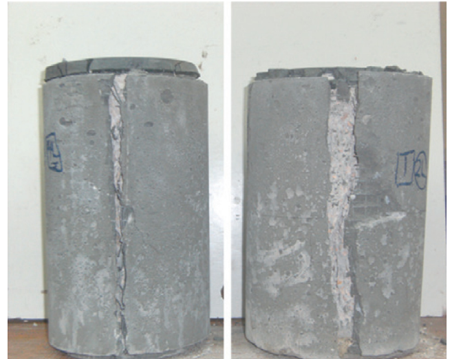
Fig. 1. Crack pattern of specimens [37].
