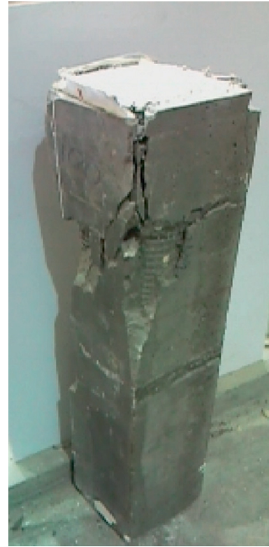
Fig. 3. Failure mode of the repaired columns [47].
