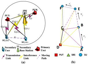
Figure 1. Mobile CRN system model.
