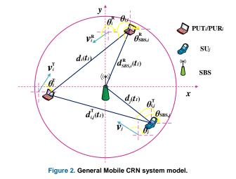
Considering the model more simply and practically, the speeds of PUs are assumed as relatively low compared with the SUs'. Thus, the shadow fading for PUs is assumed fixed during a SU's slot. Otherwise, a similar compensation parameter *SL*' will be used to predict the primary CSI:
