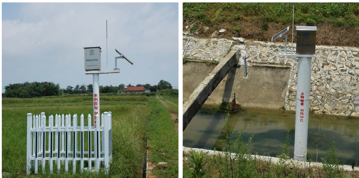
Fig. 5. Real-time In-field monitoring station examples: left, soil moisture monitor; right, canal water level monitor.
