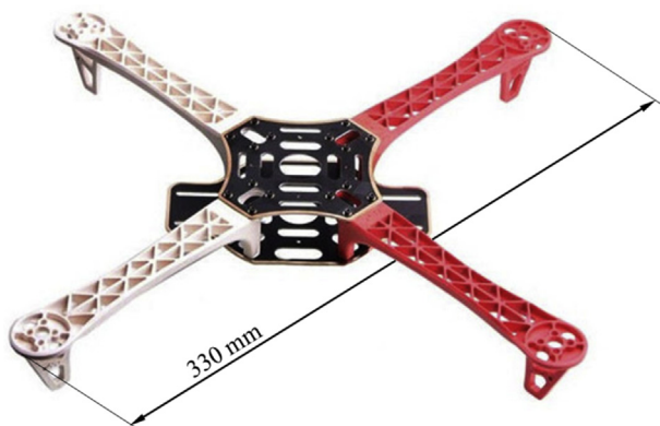
Fig. 4. Support frame of the designed SUAS.
