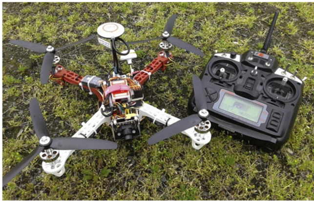
Fig. 9. General view of the designed aerial multicopter platform prototype as a part of the small unmanned aircraft system (SUAS) with the manual controller console.
