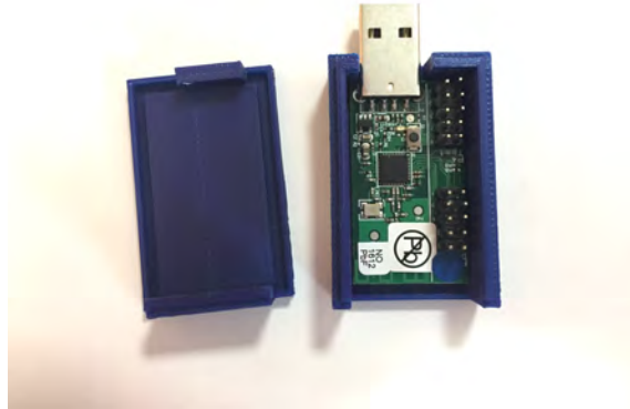
Figure 4: Example of a small USB receiver suitable for operations in the absence of power supply. The dimensions are 3 cm \times 4.5 cm
