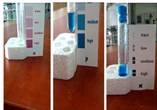
Figure 5. Nutrient content for polluted sample through thermic decontamination: a) Nitrogen – trace; b) Phosphorous – medium-high; c) Potassium – medium
