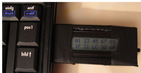
Fig. 6. Prototype of the hPIN/hTAN.
