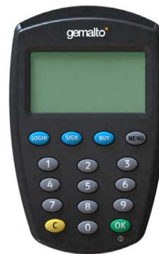
Fig. 5. A USB smart card reader with its own display and keypad.
