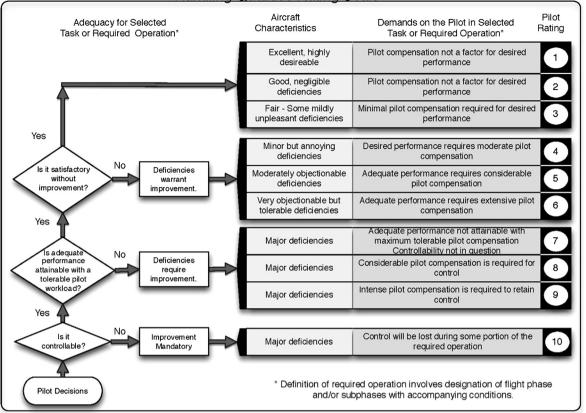
Fig. 3. The Cooper-Harper rating scale [20].
