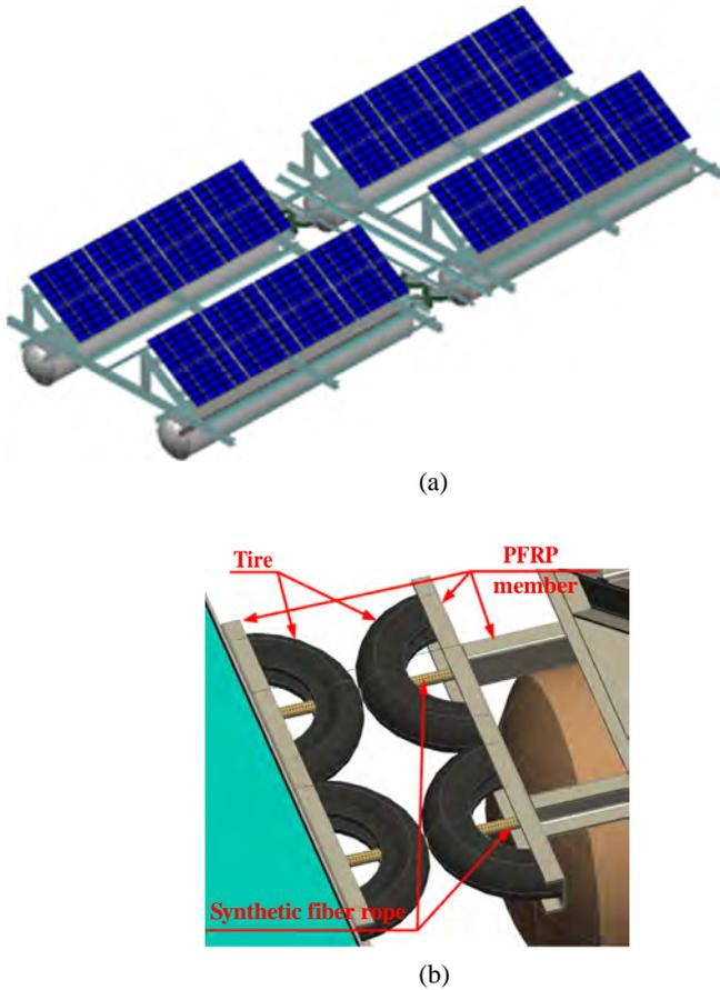
Fig. 5. Connection between unit structures. (a) ISO-view and (b) detailed view.
