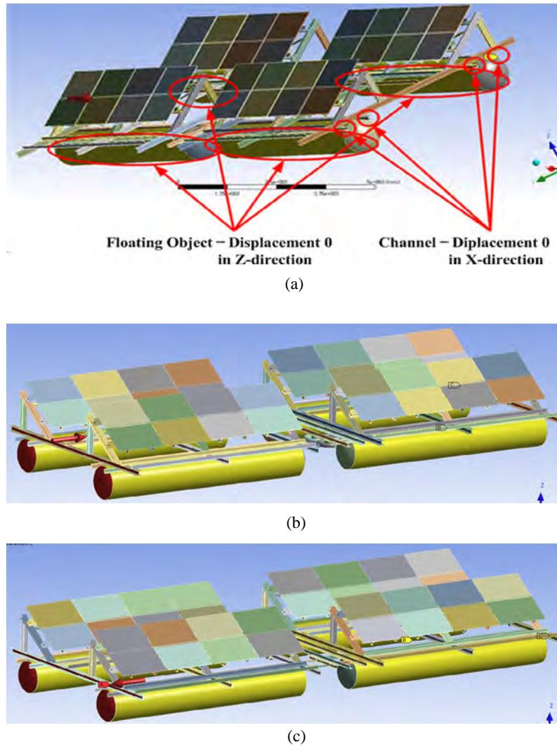
Fig. 7. Boundary and loading conditions of the connection part between modules. (a) Boundary conditions of the connection part between modules; (b) Case 1 – loading condition (compression) and (c) Case 2 – loading condition (tension).
