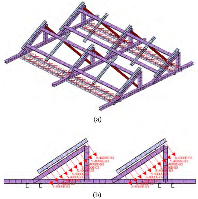
Fig. 6. Boundary and loading conditions. (a) Boundary conditions (all hinges) and (b) loading conditions.
