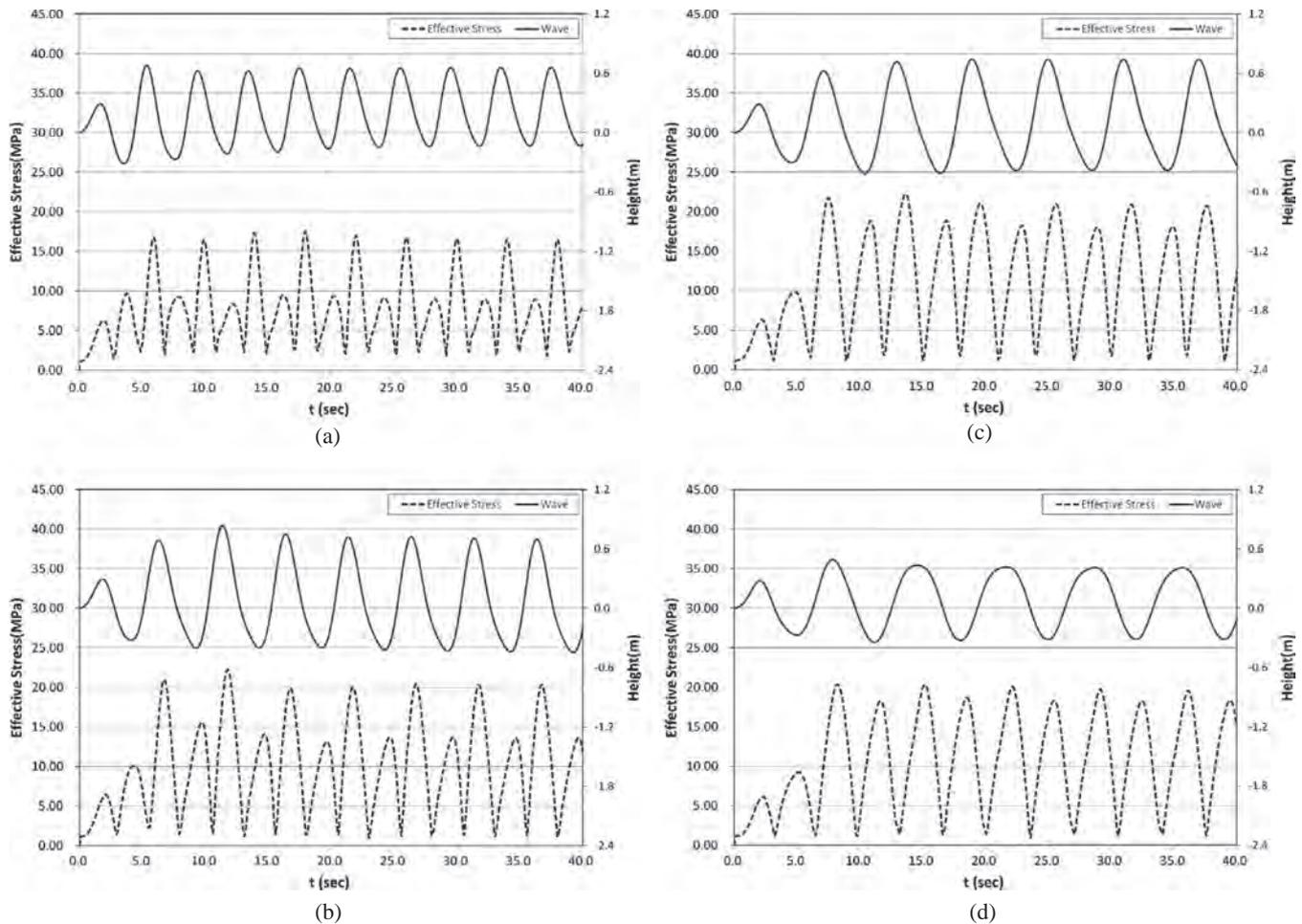
Fig. 13. Maximum effective stress in floating body for wave propagation. (a)  $T = 4$  s; (b)  $T = 5$  s; (c)  $T = 6$  s and (d)  $T = 7$  s.
