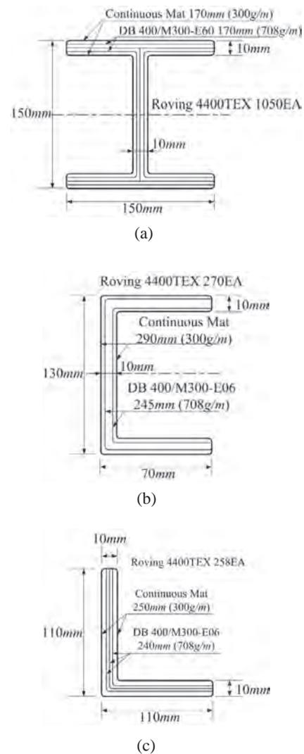
Fig. 1. Arrangement of reinforcing fiber used for manufacture and dimension of cross-section of PFRP member. (a) I-shape; (B) channel and (c) angle.
