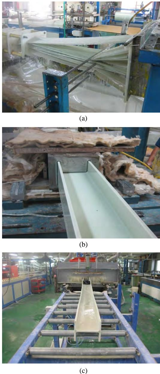
Fig. 14. Member production by the pultrusion process. (a) Fiber supply and impregnation; (b) pulling; (d) hardening.
