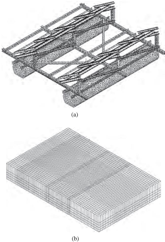
Fig. 10. Generated mesh of structure and fluid. (a) Floating structure and (b) fluid.
