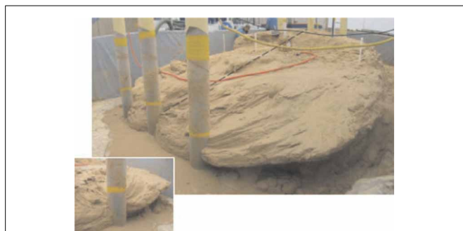
FIGURE 4 | Image of a cemented sand body from a large scale biogrout experiment. Van Paassen et al. (2010).
