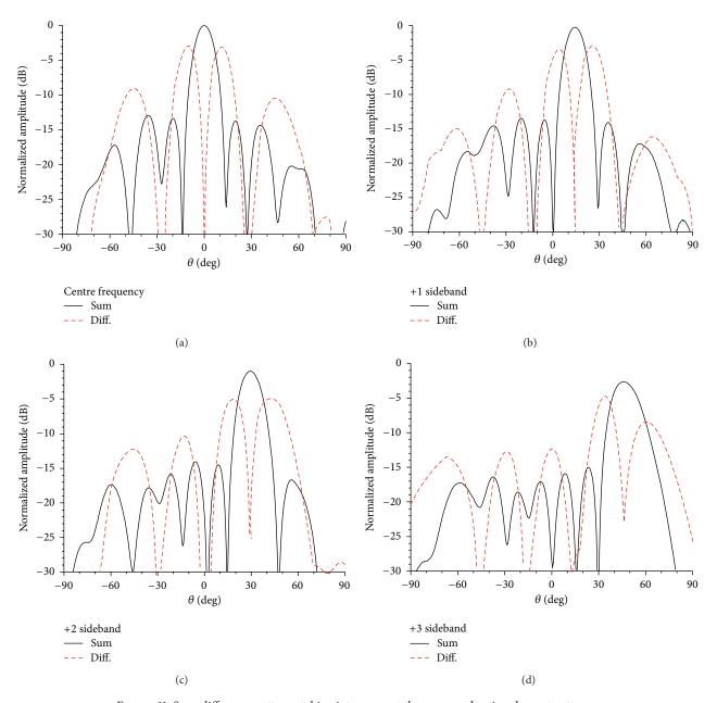
FIGURE 11: Sum-difference patterns taking into account the measured active element patterns.
