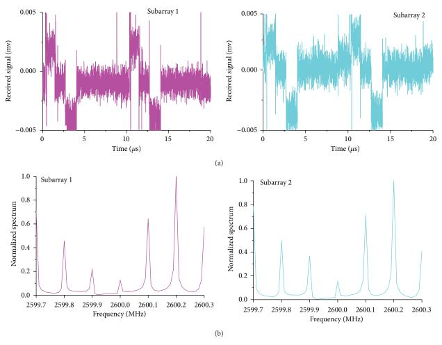
FIGURE 14: The procedure to determine the pair of sum-difference patterns that has the maximum amplitude response and should be used for angle measurement. (a) The waveforms of signals received by the two subarrays at  $\theta = 30^{\circ}$ . (b) The spectra of received signals received at  $\theta = 30^{\circ}$ , which are obtained by FFT performed in PC.
