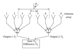
FIGURE 1: A phase-comparison monopulse system based on a conventional 8-element array.
