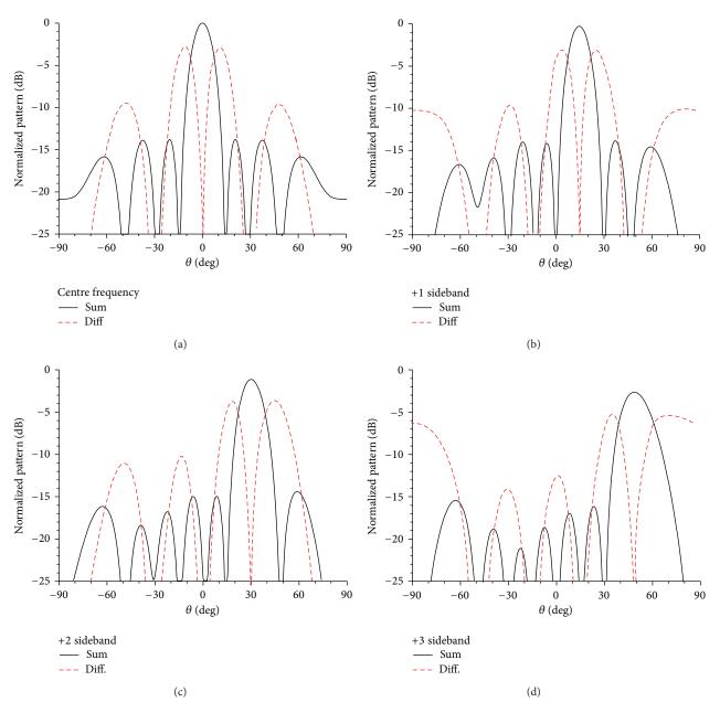
FIGURE 8: The sum-difference patterns formed at different sidebands and different pointing directions by phase-comparing the multibeams of subarray 1 and subarray 2 (only the positive sidebands are shown).
