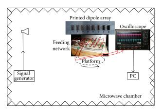
FIGURE 9: Block diagram of the experiment setup.
