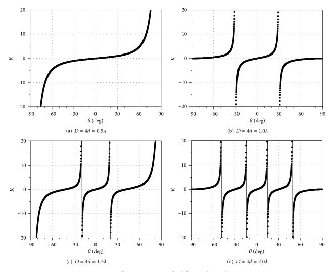
Figure 2: Difference-sum ratio *K* for different subarray distance.
