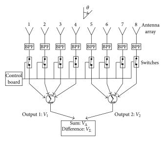
FIGURE 4: A phase-comparison monopulse system based on an 8-element 4D antenna array.
