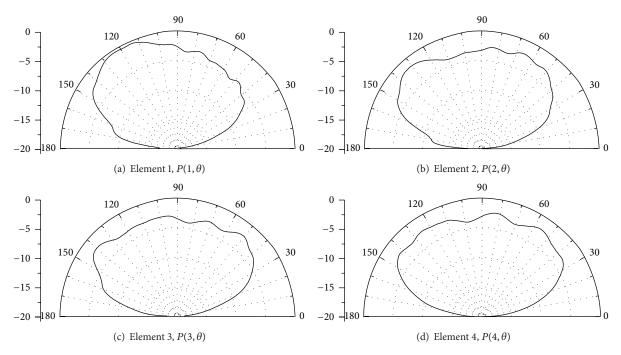
FIGURE 10: Measured normalized active element amplitude patterns of subarray 1 [denoted as  $P(k, \theta)$ ].
