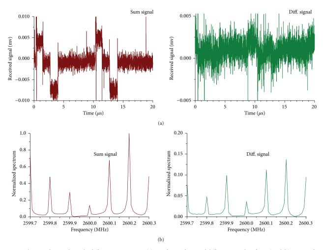
FIGURE 15: The procedure to obtain the difference-sum ratio K: (a) waveforms of sum and difference signals at  $\theta = 30^{\circ}$  and (b) spectra of sum and difference signals at  $\theta = 30^{\circ}$ .
