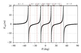
FIGURE 5: Difference-sum ratio  $K_{\rm 4D}$  of the 4D array where isotropic elements are used. For a signal coming from the mth sector,  $K_{\rm 4D}(m)$  is used.
