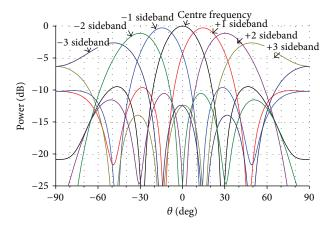
FIGURE 7: The multiple beams generated by subarray 1 and subarray 2 at different sidebands with different pointing directions.
