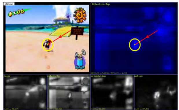
Fig. 2. Neuromorphic Vision C++ Toolkit (iNVT) developed at iLab, USC, http://ilab.usc.edu/toolkit/ . A saccade is targeted to the location that is different from its surroundings in several features. In this frame from a video, attention is strongly driven by motion saliency.
