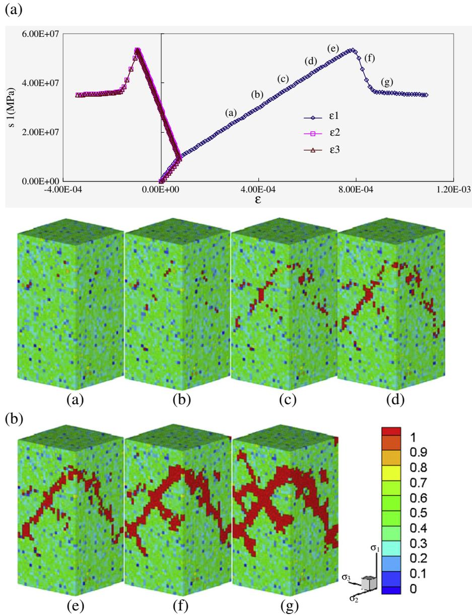
Fig. 6. EPCA3D simulated results when  $\sigma_2 = \sigma_3 = 10$  MPa using the Drucker–Prager criterion (a) relation of  $\varepsilon_1$ ,  $\varepsilon_2$  and  $\varepsilon_3$  with respect to  $\sigma_1$  (b) failure process.
