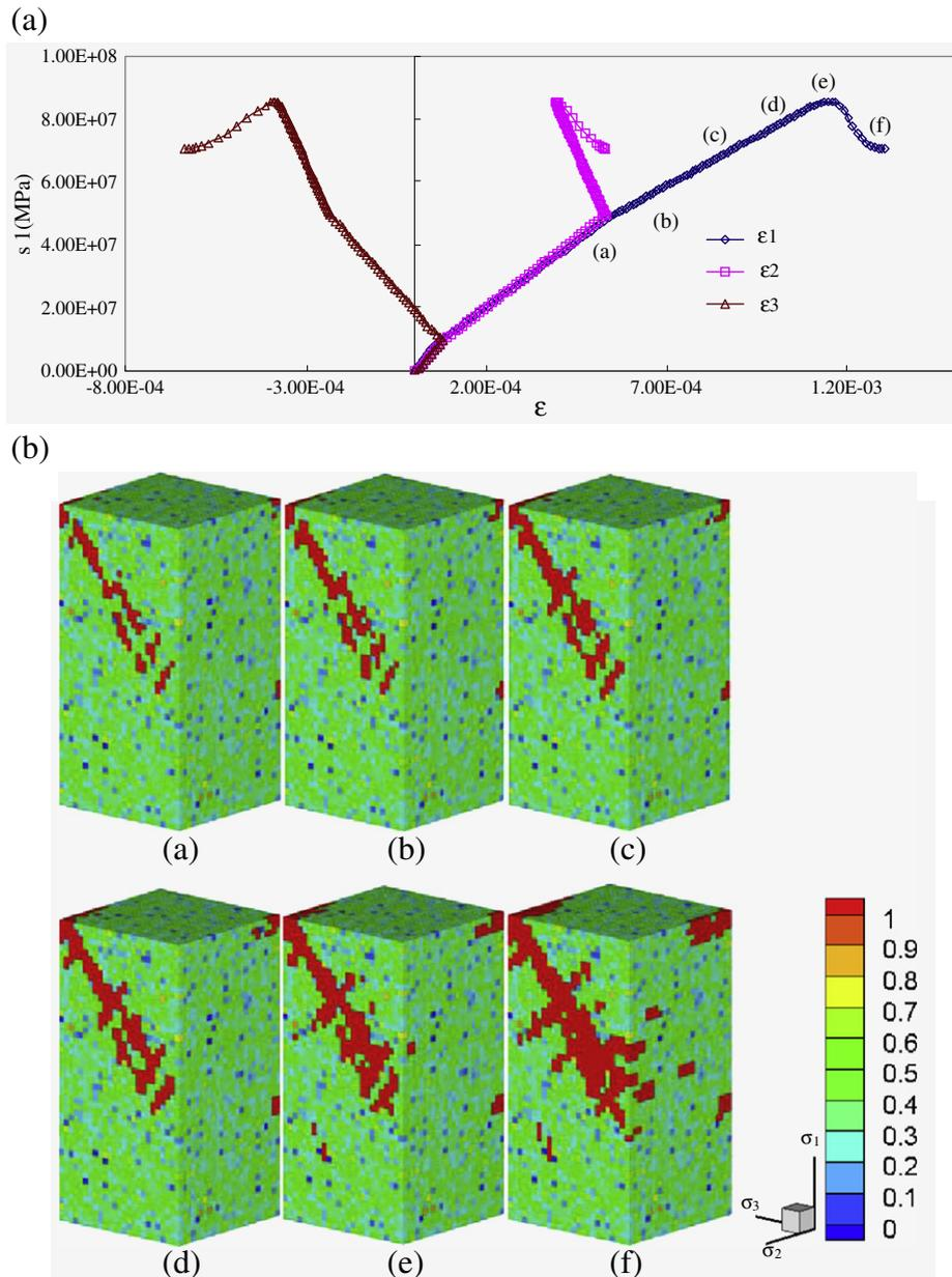
Fig. 7. EPCA3D simulated results when  $\sigma_2 = 50$  MPa,  $\sigma_3 = 10$  MPa using the Drucker–Prager criterion (a) relation of  $\epsilon_1$ ,  $\epsilon_2$  and  $\epsilon_3$  with respect to  $\sigma_1$  (b) failure process.
