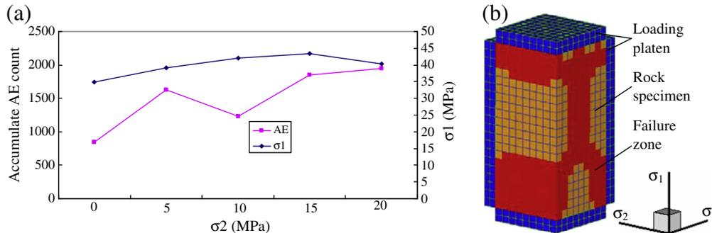
**Fig. 14.** EPCA3D simulated results when  $\sigma_3 = 0$  MPa by consideration of the loading platen effect for a homogeneous rock specimen. (a) Relation of  $\sigma_1 - \sigma_2$  and  $\sigma_2$ -accumulated AE counts before the peak stress and (b) Failure pattern (blue colour represents loading platens, orange colour represents rock specimen, red colour represents failure zone).
