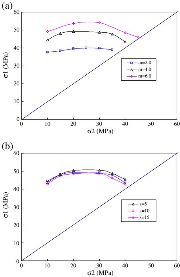
**Fig. 13.** Relation of  $\sigma_1 - \sigma_2$  with different heterogeneity ( $\sigma_3 = 10$  MPa). (a) different homogeneous indices,  $m = 2.0, 4.0, 6.0$ . (b) the same homogeneity index  $m = 4.0$ , different spatial random seed,  $s = 5, 10, 15$ .
