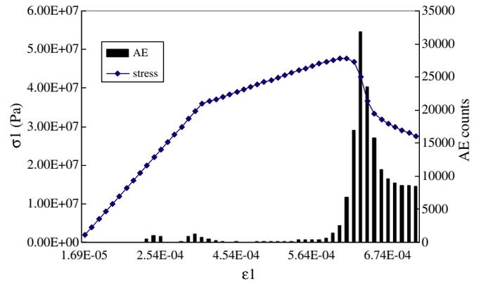
Fig. 11. EPCA3D simulated complete  $\sigma_1 - \epsilon_1$  and AE  $-\epsilon_1$  relation during the failure process modelling of heterogeneous rock using the Mohr–Coulomb criterion ( $\sigma_2 = 35$  MPa and  $\sigma_3 = 10$  MPa).
