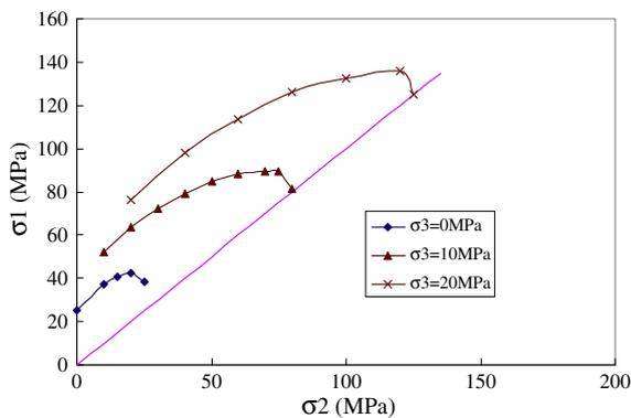
Fig. 8. EPCA3D simulated results using Drucker–Prager criterion.
