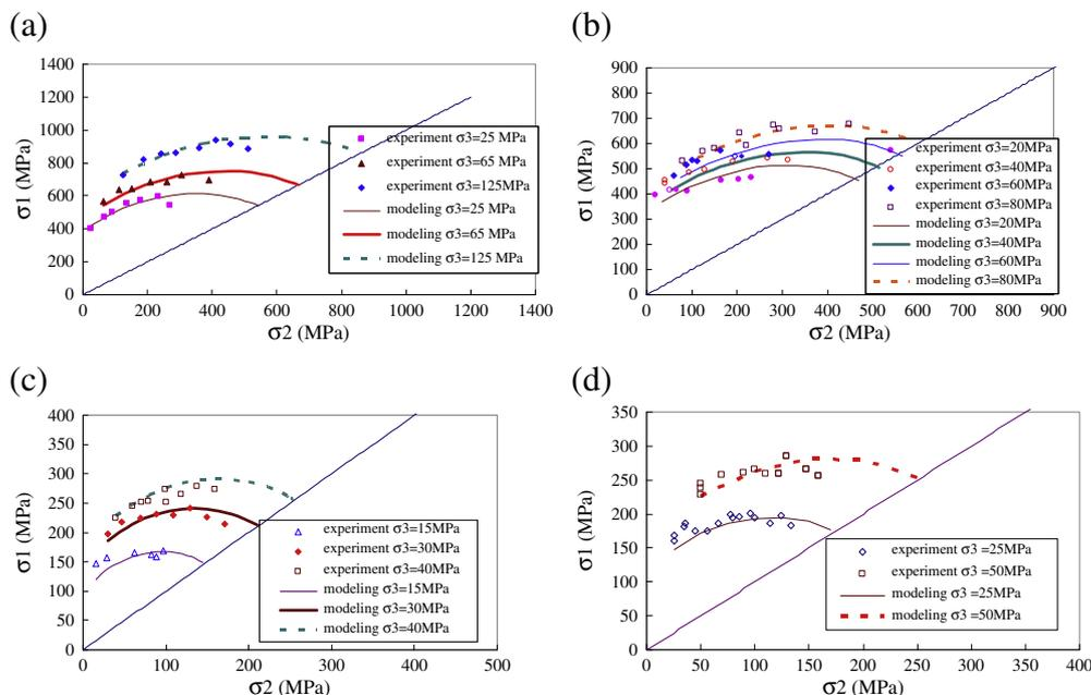
Fig. 4. The relation between  $\sigma_2$  and  $\sigma_3$  of different rock types (curves are EPCA3D results. Discrete points are experimental results). (a) Dunham dolomite; (b) Solenhofen limestone; (c) Shirahama sandstone and (d) Yuubari shale.
