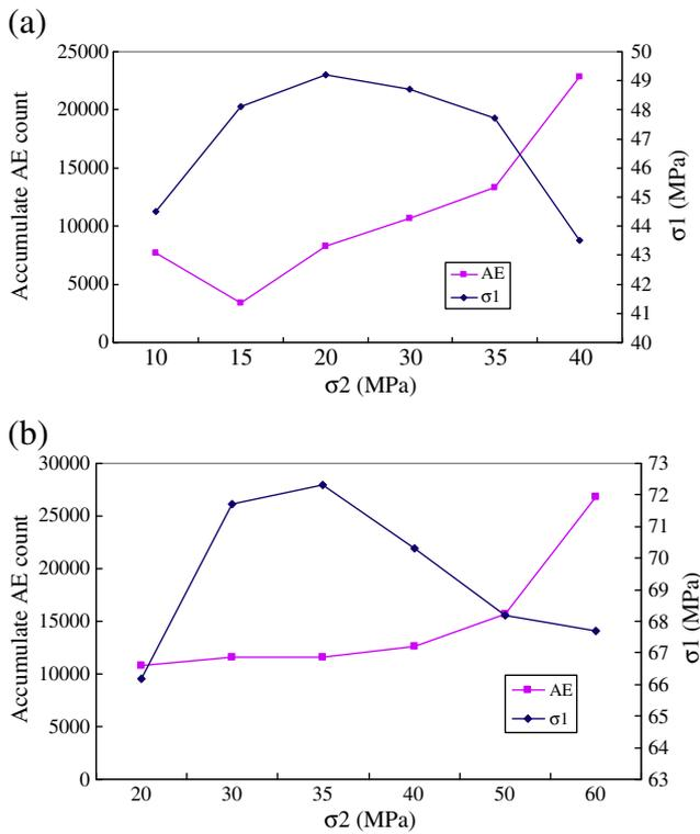
Fig. 9. EPCA3D simulated  $\sigma_1$  and accumulated AE counts before the peak stress with respect to  $\sigma_2$  using the Mohr–Coulomb criterion. (a)  $\sigma_3 = 10$  MPa and (b)  $\sigma_3 = 20$  MPa.
