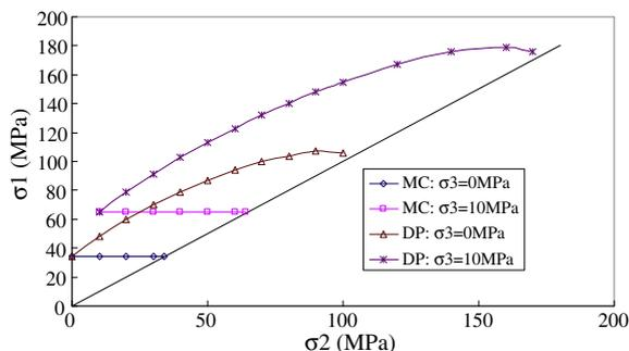
**Fig. 5.** EPCA3D simulated results for the relation between  $\sigma_1$  and  $\sigma_2$  for a homogeneous rock specimen using the Drucker–Prager criterion and Mohr–Coulomb criterion.
