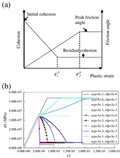
Fig. 3. (a) Cohesion weakening and friction strengthening (CWFS) model and (b) EPCA3D simulated complete  $\sigma_1 - \epsilon_1$  curves by considering different combinations of  $\epsilon_c^p$  and  $\epsilon_f^p$  in the CWFS model.
